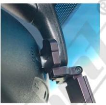
**STEP 4 -** Rotate the mount so it is parallel with the bottom of the mirror. Tighten the clamp screw untill the mount is securely attached to the mirror stem.
