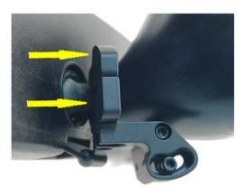
STEP 3 - When the mount is positioned as far forrward as it will go, tighten the clamp screw untill the Top and Mid Sections are slightly snug around the mirror stem. You should still be able to rotate the mount.
