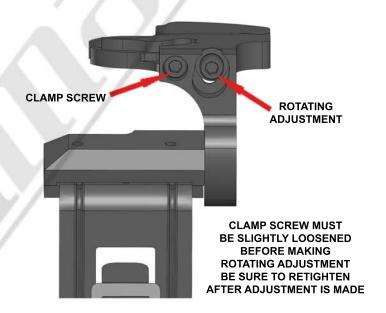
STEP 5 - Install your radar detector onto the mount. Use the adjustments shown above to adjust the RD to your desired position. We recommend adjusting the RD as close to the bottom of your mirror as you can. Be sure to tighten all adjustment screws after the adjustments are made. For the Pivot adjustment, grab the long arm of the allen wrench for maximum leverage. You will not strip the threaded holes in the aircraft grade aluminum.
